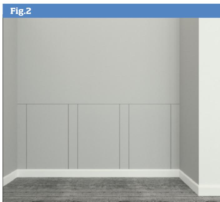
To mark horizontal lines which will locate top and bottom of panel, from distance between top of skirting and bottom of dado which is 912mm subtract height of panel 690mm = 222mm.
