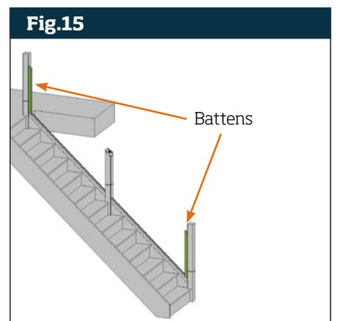
Offer handrail assembly between top and bottom newels and onto tops of battens with threaded fasteners located to side of newel faces on stair side. Mark fastener location on bottom and top newels (**Fig.16**).
