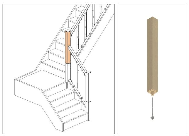
The following instructions are for installing the Cheshire Mouldings **CPSTO Storey Newel Post**. This post can be used when you have structural posts that cannot be removed eg on quarter landings and winders
