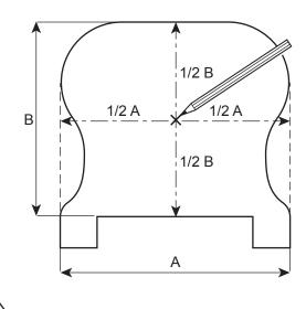
Once the handrail has been cut to the required length and at the desired angle, measure and mark the centre of the handrail. It is critical these measurements are correct to ensure an accurate fit.
