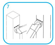
With handrail fully down onto top of glass panels, mark locations of bracket tops on top and bottom newel post faces. Remove rail and panels
