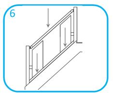
To establish handrail location, place a rake glass panel in base rail groove at bottom and top of stairs, using an 80mm timber off cut to create a gap between panel and post to accommodate connectors. Use spirit level to ensure panels are vertical. Offer handrail assembly over panel tops. This is best done with 2 people
