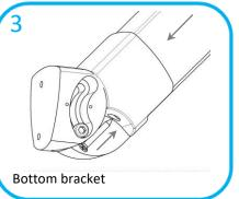
Offer handrail into bottom connector. It may be necessary to chisel the rail end slightly, in order to achieve a good fit. Pilot drill through screw hole at back of connector and secure with suitable screw
