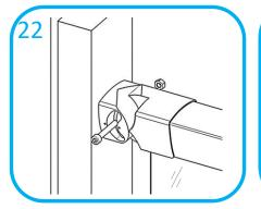
Fix rail brackets to base brackets on the posts using nuts and bolts supplied
