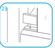
Working from one side, take handrail and base rail fillets which have been cut to suit the gap. Fit into groove using glue and screwing through (you will need to drill clearance holes through fillet) or use nail gun with suitable size nails. Push panel to fillet ends, check vertical and fix next pair of fillets. Fill any screw/nail holes with filler and sand smooth.
