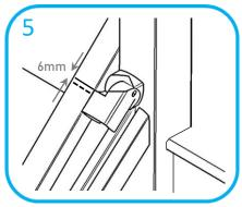
Mark the handrail in line with back of the rail connector hood as shown above. Measure and mark 6mm down from the mark and cut handrail to length. Fix top connector to top rail end (see Fig 3)
