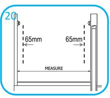
Measure distance between landing newel posts. Glass panels should be positioned no closer than 65mm away from both landing posts. Subtract 130mm from post to post measurement to give actual dimension. Follow procedure shown in italics in Fig 9
