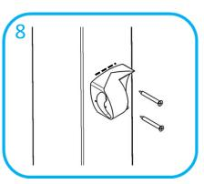
Fix bracket base part to bottom and top newel post marks, ensuring they are central to post face. Drill pilot holes and fix to newels using screws supplied
