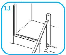
Install half newel post to wall at same height as post at top of stairs. Measure between posts and cut and fix base rail to floor, ensuring screw heads are below groove face.
