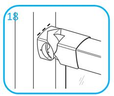
With handrail fully down onto panel tops, mark the location of the bracket tops onto both newel posts. Remove rail and panels
