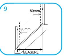
To work out how many panels are required, measure horizontal distance between posts. **NB panels should be set 80mm min from newel posts.** Subtract 160mm from post to post measurement to give actual distance. *Divide this distance by width of panel + 50mm, Round down to next whole number (panels). Multiply panel width by number of panels. Subtract this from actual distance. Divide this by number of panels minus 1 to get gap sizes eg 3 panels -1 = divide by 2*
