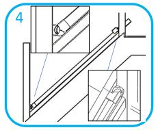
Offer bottom connector and rail assembly to bottom newel post face so handrail points up the stairs. Position top connector against top newel post so the rail runs alongside it. This requires 2 people
