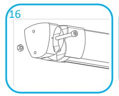
Connect base part connector to rail connector on both rail ends using nuts and bolts supplied.
