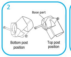
Assemble 2 off adjustable connectors using nut and bolt supplied. One will be for the bottom post with the connector facing up and one will be for top post with connector facing down
