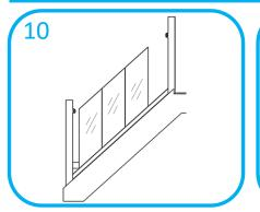
NB if gaps are greater than 99mm, add an extra panel and recalculate.
