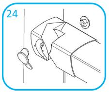
To finish, fix all cover caps in place to hide fixings. Run a small bead of clear silicon withing the bracket opening and press the cover caps into place
