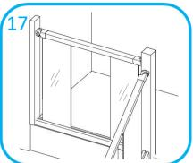
Insert 2 landing panels into the base rail groove and position them approx. 60mm away from posts at each end. Offer handrail assembly between posts and onto top of handrail so panel tops are in the rail groove.
