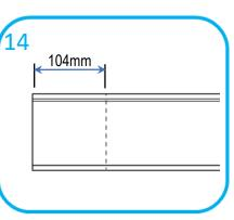
Run bead of clear silicon in handrail groove.
