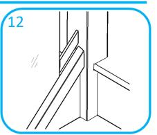
Working from top post down, take handrail and base rail fillets which have been cut to suit the gap. Fit into groove using glue and screwing through (you will need to drill clearance holes through fillet) or use nail gun with suitable size nails. Push panel to fillet ends, check vertical and fix next pair of fillets. Repeat until run is completed
