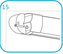
Offer rail brackets to each end of the handrail, drill pilot holes and fix using screws supplied.
