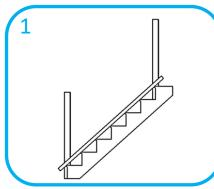
Place base rail on stair nosing and offer up to newel posts. Mark and cut to length. Fix base rail to top of string by drilling clearance hole through bottom of base rail groove and secure with suitable screws, ensuring the screw heads are sunk below groove face
