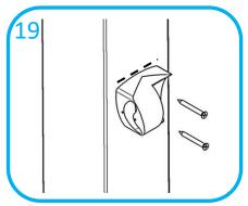
Fix bracket base part to both newel post marks, ensuring they are central to post face. Drill pilot holes and fix to newels using screws supplied
