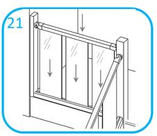
Run bead of clear silicon into base rail groove. Insert all glass panels. Run bead of clear silicon into handrail groove and carefully offer handrail assembly between posts and over panel tops.
