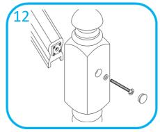
Apply some PVA glue to rail faces. Offer rail between newels so insert plates locate into recesses in newel face. Offer bolt and washer through hole and tighten to secure rail to newel. Apply some PVA glue to cover cap and gently tap into hole to hide bolt head.
