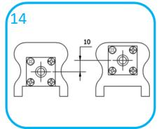
For situations where the landing has a corner newel, position insert plates on cut ends of handrails so one is positioned near the top of cut face and one is positioned near bottom of cut face so they are staggered 10mm minimum
