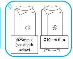
Using a Ø25mm flat bit, drill a hole to a depth of 23mm for 90mm square newels or 15mm depth if using 82mm square newels. Next, drill a Ø10mm hole through, ensuring that the drill is kept level and straight.
