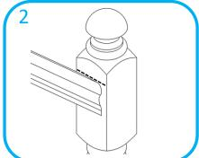
After handrail has been cut to length, place between stair newels at required height and mark top of handrail locations on both bottom and top newels. Please note – top of handrail must be set at least 900mm high (above pitch line)
