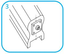
Place fixing insert plate on cut face at bottom of rail so it is central and positioned to the upper half of the face so there is plenty of material for the fixings. Mark through 4 x screw hole and centre hole locations onto rail face
