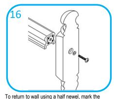
newel as previous. Drill a Ø25mm counterbore in back of half newel to a depth of 10mm then a Ø10mm hole through. Cut the bolt to length so when it is inserted into the hole, it projects approx. 10mm through. Secure rail to newel then fix half newel to wall. Fill any screw holes with filler or use flush pellets to hide screw heads.
