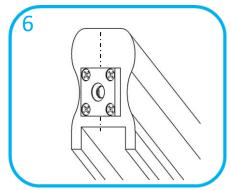
Repeat steps for top cut face but this time place the fixing insert plate to the bottom half of the face
