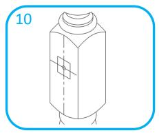
Where the Ø10mm hole exits on the rail face of the newel, draw centrelines across hole location and offset these lines by 16.5mm to create a square 33mm x 33mm central to the hole
