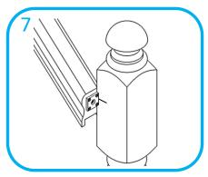
Place handrail between stair newels with insert plates pushed up to side face of newels. Check that the top of the handrail is aligned with height location marks set out in Fig 2. Mark mid point of insert plate onto side face of newels
