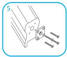
Offer fixing insert plate to rail face so the threaded centre boss locates within 13mm hole. Line up screw holes with pilot holes. Using the screws supplied, fix to rail end.
