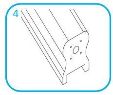
Use a 2mm drill bit to pilot drill the 4 x screw holes to a depth of 25mm. For the centre hole, use a 13mm drill bit to a depth of 14mm
