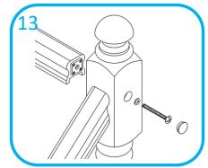
For landings, measure and cut all handrails to length. Mark handrail top positions on all newel faces (900mm high minimum). Follow same procedure as used on stairs for marking and drilling fixing holes on newels.
