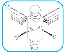
Offer handrail with plate inserts to side of corner newel so tops of handrails are aligned with height location marks. Follow same procedure used on stairs for marking and drilling fixing holes on newel. Fix rail to newel using bolt and washer
