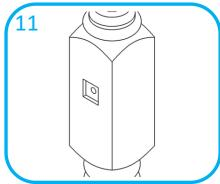
Using a sharp chisel, cut out the 33mm square to a depth of 6mm. Repeat actions for top newel
