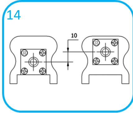
For situations where the landing has a corner newel, position insert plates on cut ends of handrails so one is positioned near the top of cut face and one is positioned near bottom of cut face so they are staggered 10mm minimum
