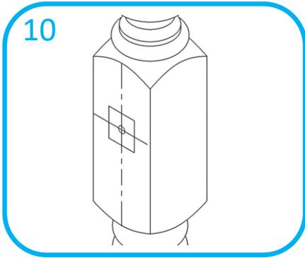
Where the  $\text{\O}10\text{mm}$  hole exits on the rail face of the newel, draw centrelines across hole location and offset these lines by 16.5mm to create a square 33mm x 33mm central to the hole
