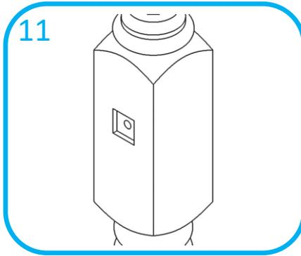
Using a sharp chisel, cut out the 33mm square to a depth of 6mm. Repeat actions for top newel
