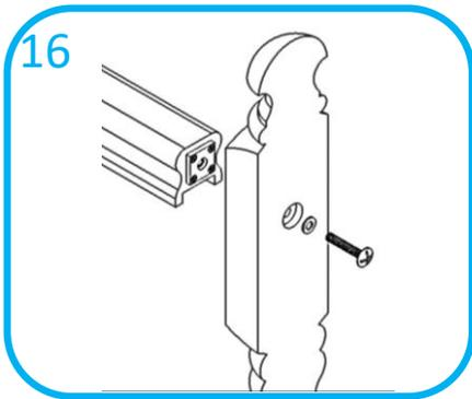
To return to wall using a half newel, mark the newel as previous. Drill a  $\text{\O}25\text{mm}$  counterbore in back of half newel to a depth of 10mm then a  $\text{\O}10\text{mm}$  hole through. Cut the bolt to length so when it is inserted into the hole, it projects approx. 10mm through. Secure rail to newel then fix half newel to wall. Fill any screw holes with filler or use flush pellets to hide screw heads.
