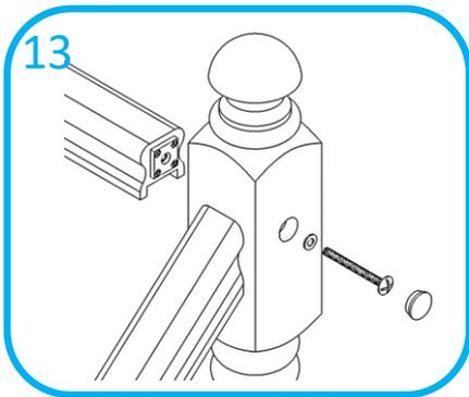
For landings, measure and cut all handrails to length. Mark handrail top positions on all newel faces (900mm high minimum). Follow same procedure as used on stairs for marking and drilling fixing holes on newels.
