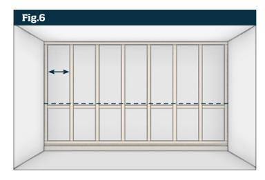
Next, measure the internal height and width of each panel square/rectangle. Cut panel moulds to length with mitred corners (**Fig 7**).
