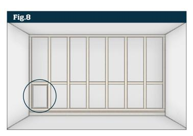
Repeat for each panel until all panel mouldings are fitted and secured (Fig 9).
