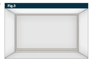
Mark centre locations of side panel strips where they join top and bottom strips. Measure distance between centres and divide by preferred number of panels going across.
