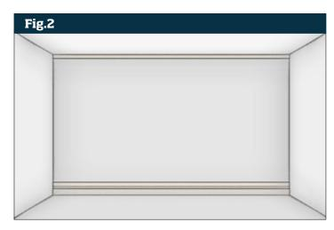
Measure, mark and cut strips for left and right sides. Check level and install as before (**Fig 3**).
