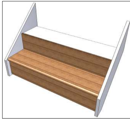
Fig. 6 The first tread assembly should look like this, and now continue up the stairs fitting a riser first followed by the tread.
