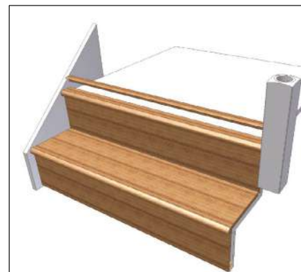
Fig. 9 Once you reach the top of the stairs, first establish the type of flooring you wish to join the cladding to, and then purchase an appropriate threshold (available in store) which will then bridge the joint between the two types of flooring. You will have to cut to top tread back so that it is level with the newel post.
