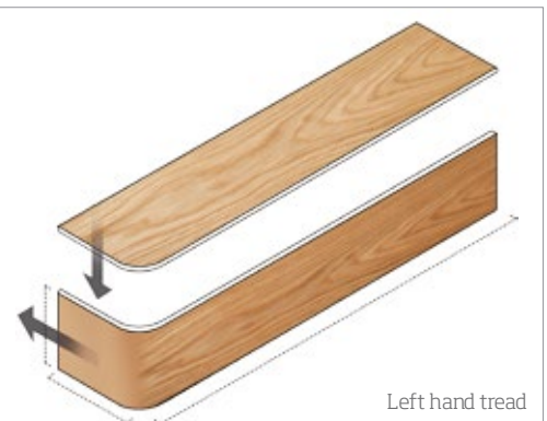
Fig. 9 Once you reach the top of the stairs, first establish the type of flooring you wish to join the cladding to, and then purchase an appropriate threshold (available in store) which will then bridge the join between the two types of flooring. You will have to cut to top tread back so that it is level with the newel post.
