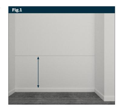
Measure length of wall (example shown is 2m). The panels when assembled measure 515mm wide x 690mm high (**Fig 2**).
